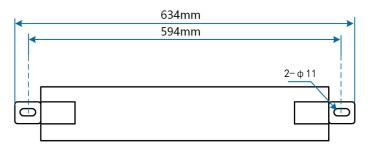
figure 4-1 Dimensions of mounting-bracket
