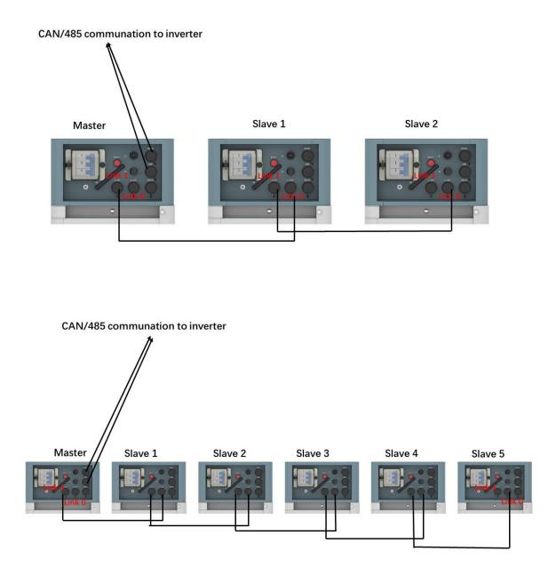
The communication for master/slave string connection shall use a 8pin pin-pin RJ45 cable, connecting from first BMS Link 1 to second BMS Link 0, then from second BMS Link 1 to third BMS link 0(if has), all the way to the last BMS Link 0. The BMS with Link Port 0 EMPTY is defined as the Master string, which further communication with the inverter or upper controller.
