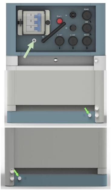
Grounding cable must  $\geq$  10AWG. The cable shall be copper with yellow-green color.
