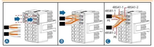
• Connect the RS485 communications cable to the power meter.
