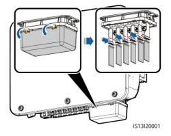
2. Connect the AC output power cable (using a five-core cable as an example).
