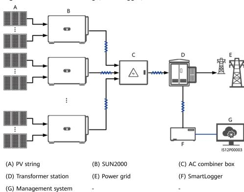
Figure 5-3 MBUS networking (SmartLogger)
