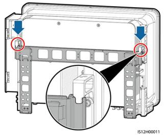
**Step 5** Secure the solar inverter.
