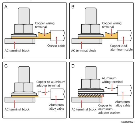
Figure 5-13 Requirements for the OT/DT terminal
