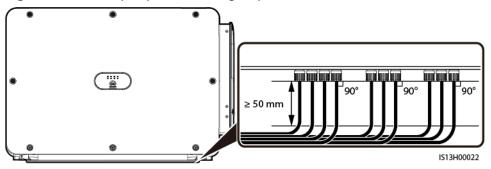
Figure 5-25 DC input power cabling requirement
