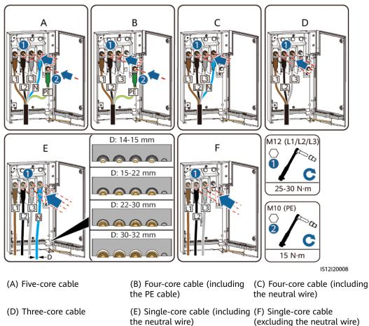
Figure 5-17 Cable connections
