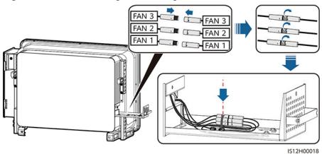
Figure 8-15 Reconnecting and binding the cables
