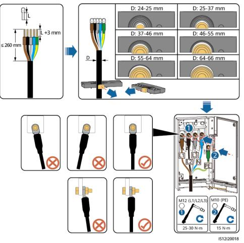
Figure 5-15 Multi-core cable connections
