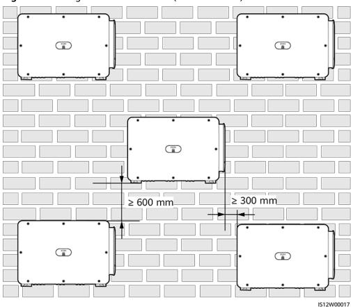
Figure 4-5 Triangle installation mode (recommended)
