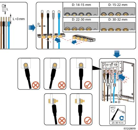
Figure 5-16 Single-core cable connections
