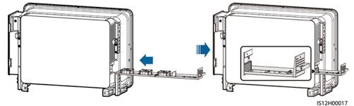
**Step 9** Connect the cables correctly according to the cable labels and bind the cables.
