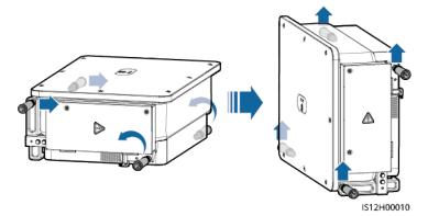
Figure 4-14 Lifting the solar inverter and keeping it upright
