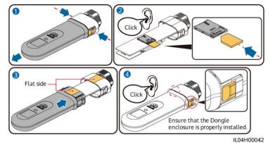
**Step 2** Secure the Smart Dongle.
