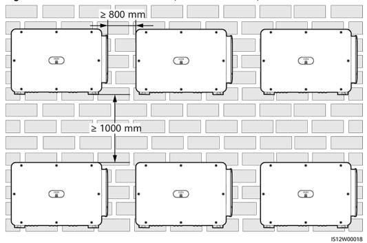
Figure 4-6 Stacked installation mode (not recommended)
