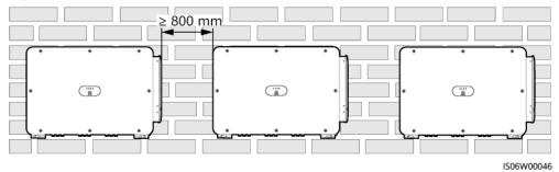
Figure 4-4 Horizontal installation mode (recommended)
