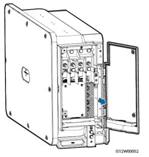
**Step 3** Select a crimping module according to the type of the AC output power cable.
