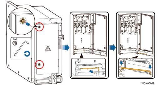
Figure 5-7 Opening the maintenance compartment door
