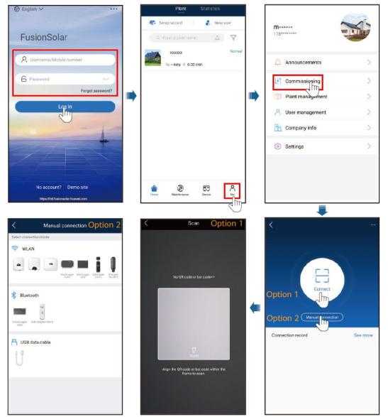
Figure 7-4 Selecting a connection mode (with network access)
