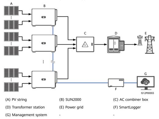
Figure 5-1 RS485 networking (SmartLogger)
