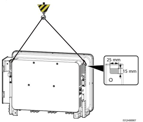
Figure 4-15 Hoisting the solar inverter
