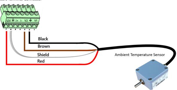
Figure 4: Connecting the Ambient Temperature Sensor
