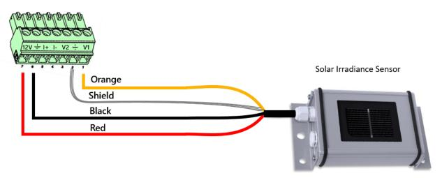
Figure 8: Connecting the Solar Irradiance Sensor
