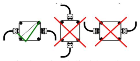
Figure 7: Correct mounting orientation of the Module Temperature Sensor
