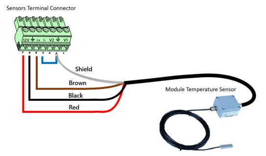
Figure 6: Connecting the Module Temperature Sensor
