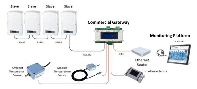
Figure 1: Commercial Gateway Connected to 3 Sensors
