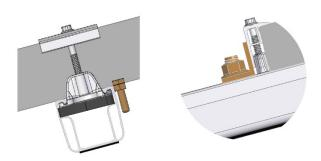
Prior to mounting modules in portrait, the module slip guards must be fitted to the frame holes above the top and bottom rail position (MV 2). For mounting modules in landscape module slip guard sets must be inserted at the lowest module row.
