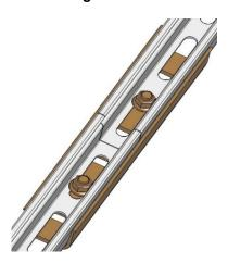
Place the rail on module supports. Position the elongated hole of the rail over the bolt in the support. Secure the rail to each module support using the M12 flange lock nut.
