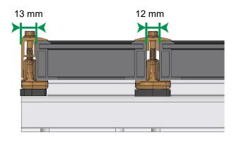
End clamps may be mounted flush with the rail end.
