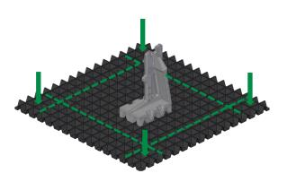
Position module supports (high/low) on the substrate plates according to the planning documents.
