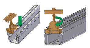
At the clamping point, guide the middle and end clamps into the rail chamber from the top. Then turn the rail nut inside the rail and push the module clamps onto the module frame.
