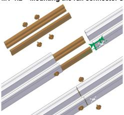
MV 1.3 - Mounting the floating bearing C-rails
