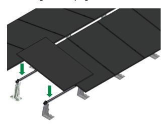
Position the photovoltaic modules upright onto the mounting rails, ensuring that they are straight. End clamps are used at the start and the end of a module row; middle clamps are used between the modules.
