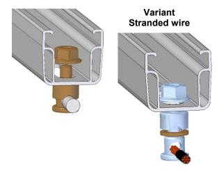
Grounding wire ( $\varnothing$  as per national specifications): Disassemble grounding connector, remove clamp washer. Push the component through the hole in the C-rail from below. Push the grounding wire (2) through the opening (suitable for  $\varnothing$  6–10 mm) and fasten the component to the rail floor with the serrated self-locking flange nut.
