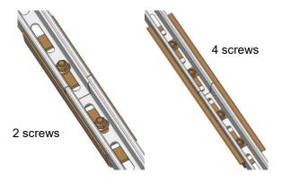
MV 1.2 - Mounting the rail connector set C47 S
