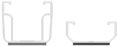
Short profile C47 with EPDM 385 mm Short profile C24 with EPDM 385 mm
